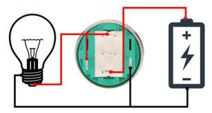
Normally closed wiring mode 2 After the power is turned on, the light is always on, and the load is powered on normally, press the button power off after pressing the button.
