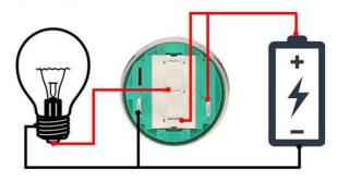
Normally closed wiring mode 1 The light on and off is controlled by the button, and the load is powered on under normal conditions. Power off when the button is pressed.
