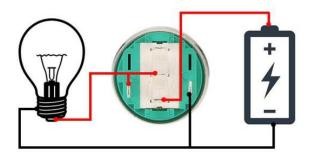
Normally open wiring mode 2 After the power is turned on, the light is always on, and the load is powered off under normal conditions. Press the button power on after pressing the button.
