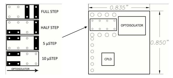
Once the jumpers have been located they may be set according to the diagram below. Please note that the four pins closest to the optoisolator are unconnected and can be used as jumper storage. It is recommended that needle nose pliers or tweezers be used to adjust the jumper settings. The power to the G210X must be turned off before any adjustment is to be made on the step pulse multiplier.
