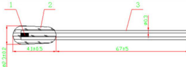
MF58J • 1---chip, 2---glass encapsulation, 3---lead wire
