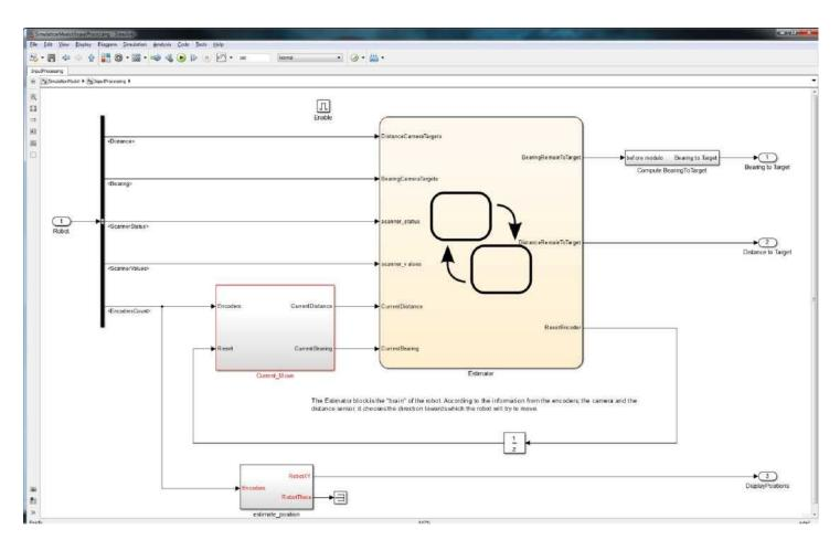
The robot's path logic is in the "Estimator" unit, shown as a Stateflow state diagram. The MathWorks Stateflow product is a decision logic modeling and simulation environment based on finite state machines.
